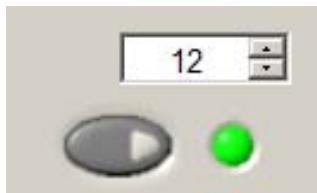
Figure 24. Calibration current enabled and directed to channel 12 of an I3200.
